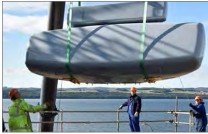
Figure 2 | This image shows the Artisan 3-D system in the process of being installed on a Queen Elizabeth Class carrier. Photo courtesy of BAE Systems.
