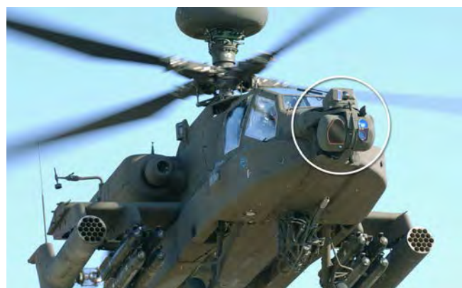
Figure 4 | M-TADS/PNVS brings color to pilots in the cockpit. Photo courtesy of Lockheed Martin.
