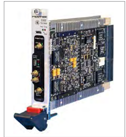
Figure 1 | The Onyx Virtex-7 Software Radio Module from Pentek for extremely wideband signal applications is based on the Xilinx Virtex 7 family and can digitize signal bandwidths up to 1,500 MHz.
