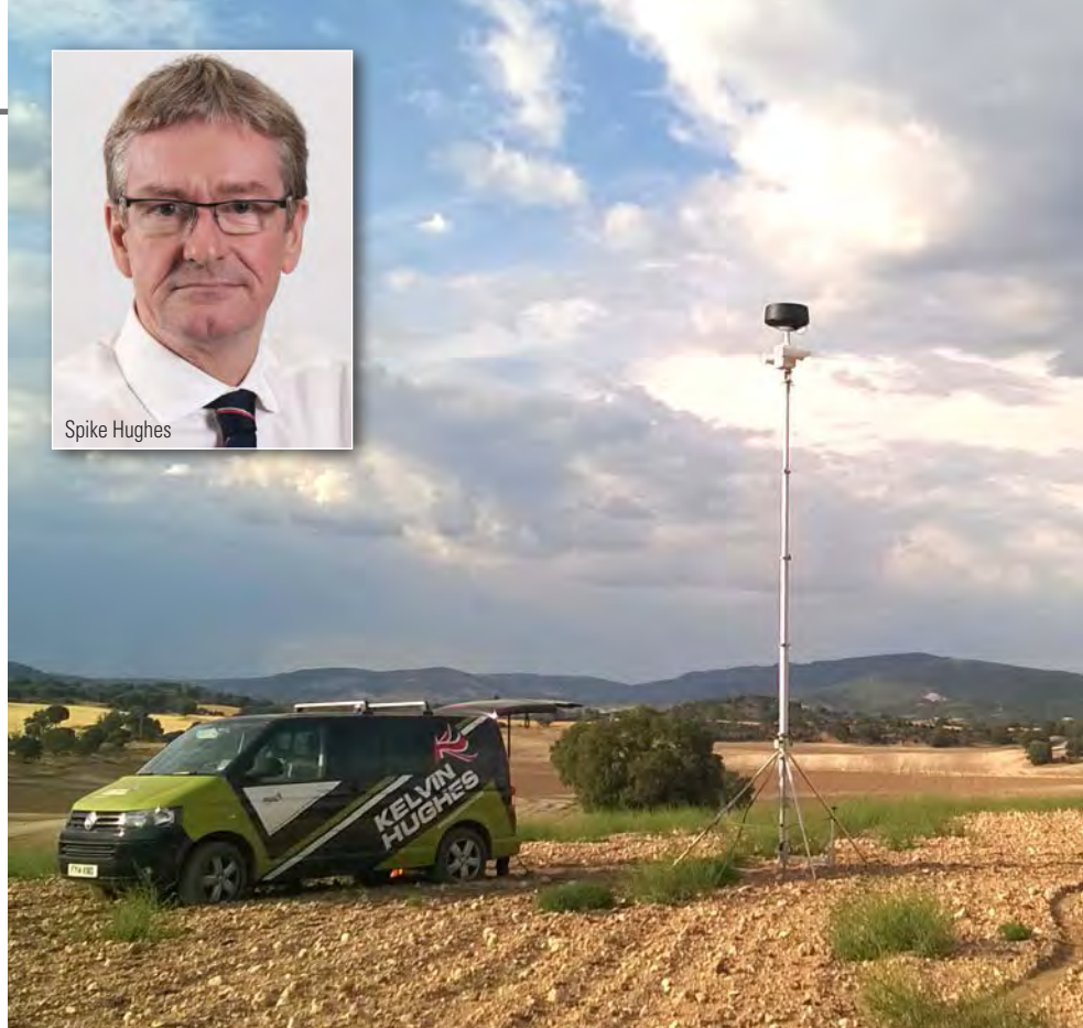
The Kelvin Hughes SharpEye SxV radar, shown in a mobile single-mast arrangement, can monitor and intercept threats from drones in remote or difficult-to-access locations. Photo courtesy of Kelvin Hughes.
