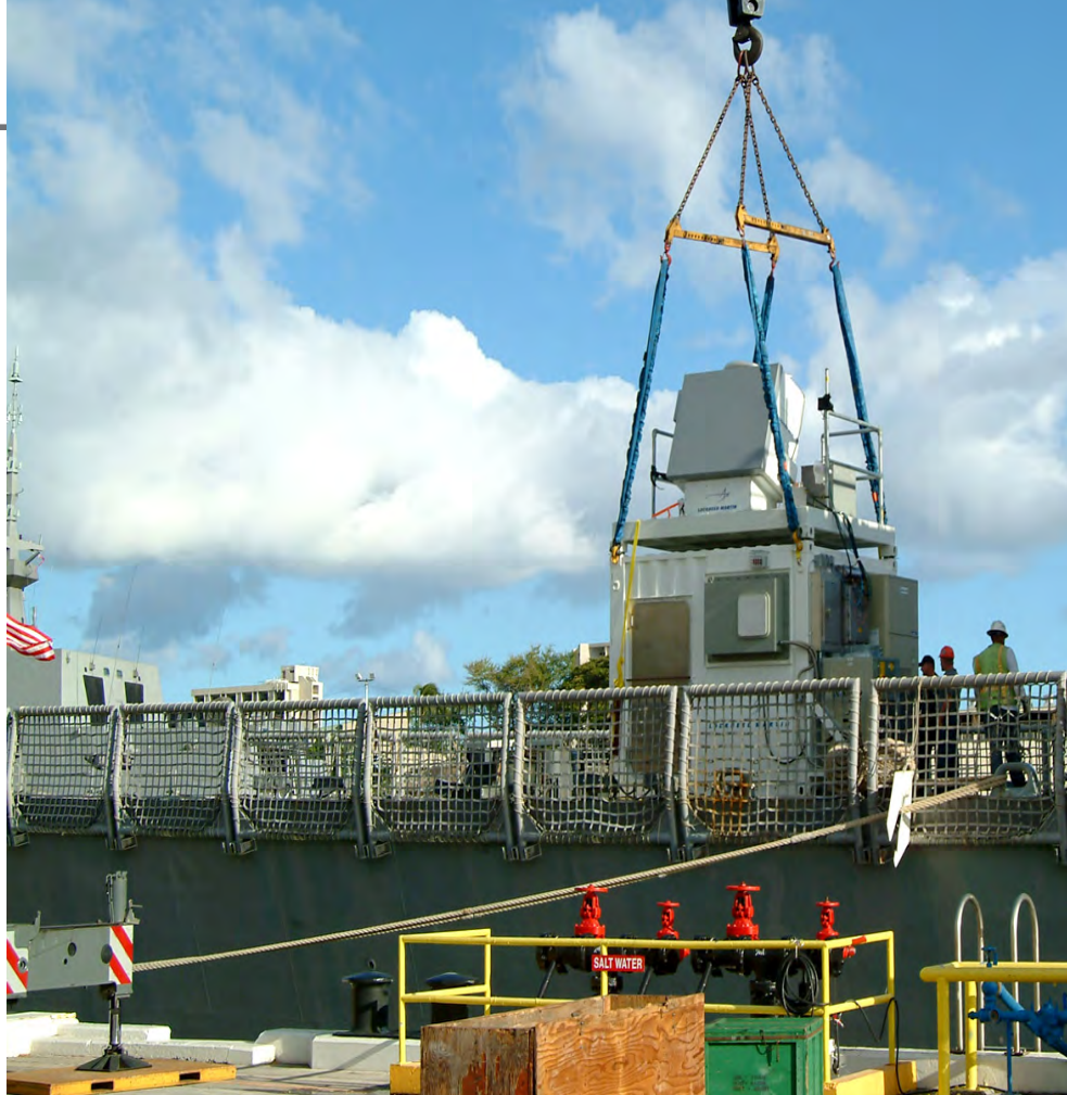
Modern electronic warfare systems such as the U.S. Navy's Surface Electronic Warfare Improvement Program (SEWIP) will rely on open architectures and commercial signal processing technology. In this photo, an early Block 3 version of SEWIP is being brought on board a Navy vessel during the multinational Rim of the Pacific (RIMPAC) maritime exercise near Hawaii in 2012. Photo courtesy of Lockheed Martin.
