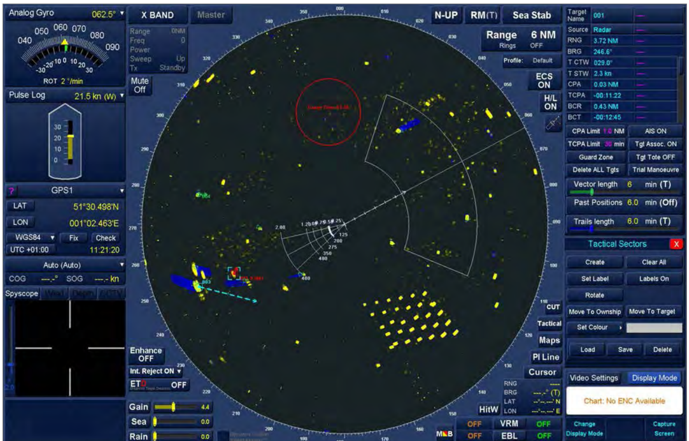
Figure 1 | An X-Band radar system display from Kelvin Hughes tracks helicopters from maritime platforms.
